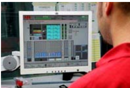
Baldwin's LithoSpray World spray bars are controlled by the existing controls in the press console.
