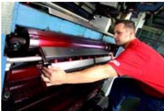
The new Baldwin LithoSpray World spray bars ensure a uniform flow of dampening solution.
