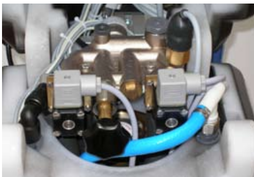
Valve block for regulation and control of the various partial flows
