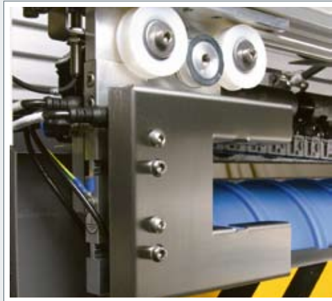
DSA-2 sensor on the exit side of the web catching system
