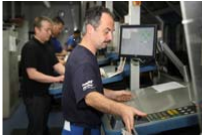
Printers at Göttinger Tageblatt can complete fine adjustments of the fountain solution supply on the press control desk.
